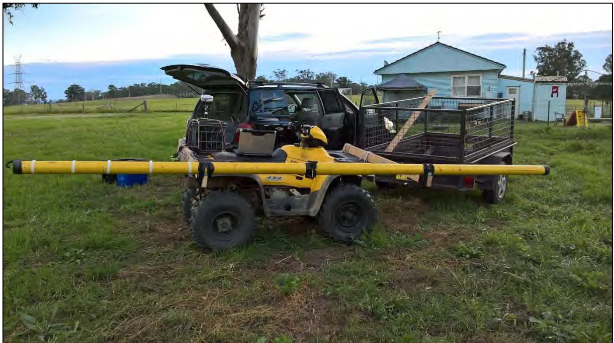
Figure B3: DUALEM Profiler extended across quad bike, with DGPS system visible at rear
